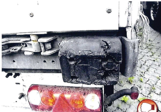
Corner bumpers Damaged corner bumpers
