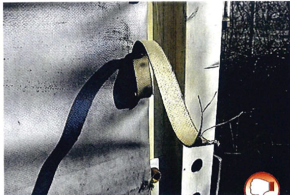
Tarpaulin strap Damaged strap (rear right side)
