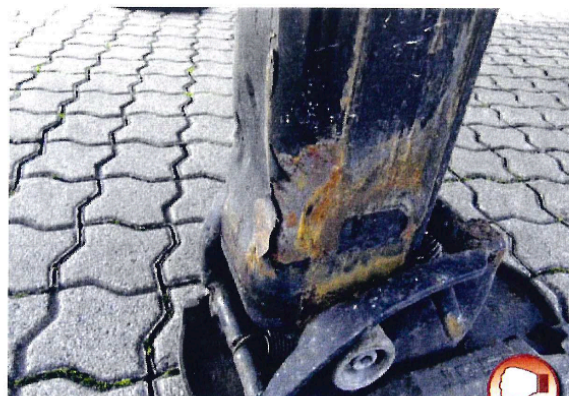
Landing gear Damaged landing gear
