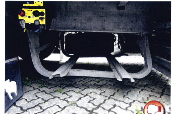
Spare wheel holder Deformed spare wheel holder
