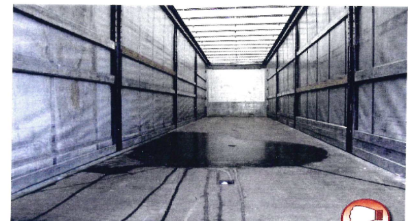
Roof tarpaulin Damaged roof tarpaulin, water puddle on the floor
