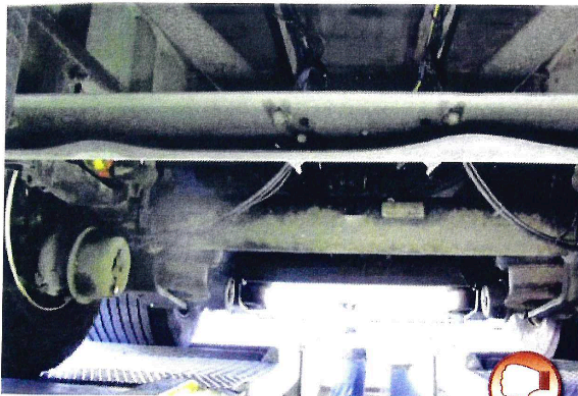
Frame cross-piece Bent frame cross-piece through wrongly positioned vehicle jack
