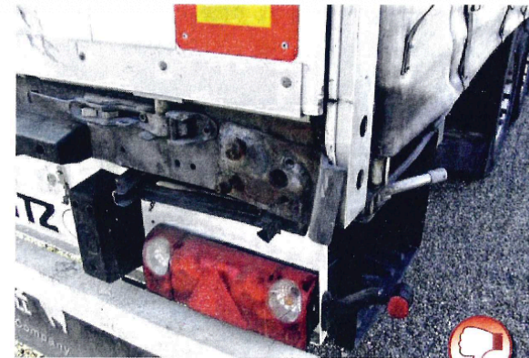
Corner bumpers Missing corner bumpers, deformed fitting
